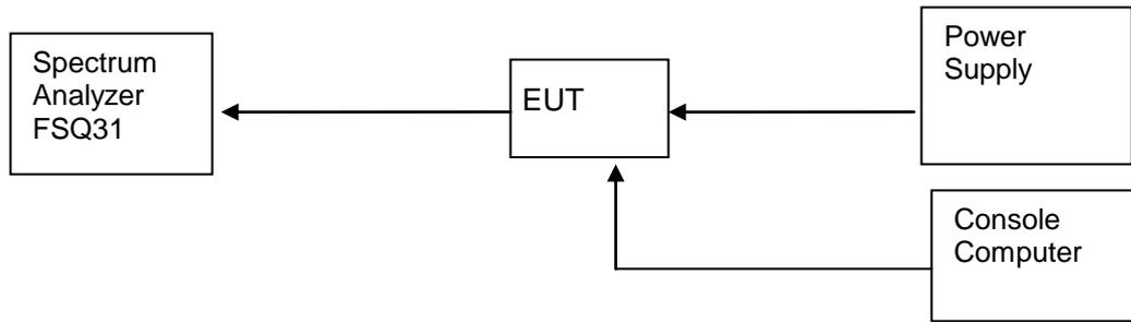
Figure 2. Test Set-up
