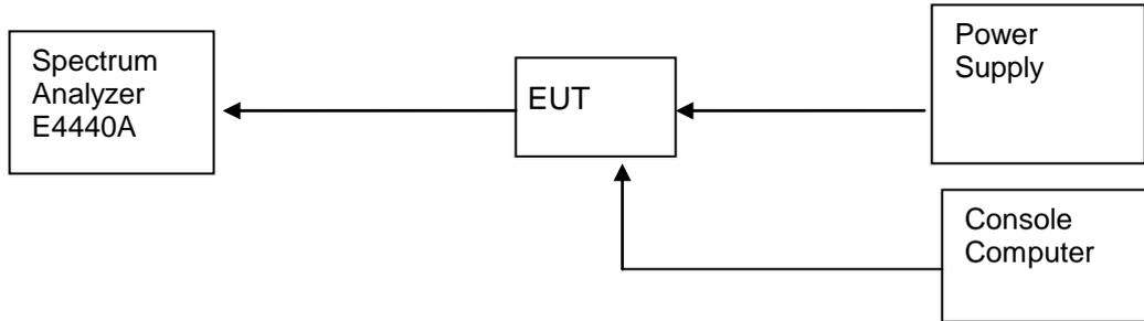
Figure 5. Test Set-up
