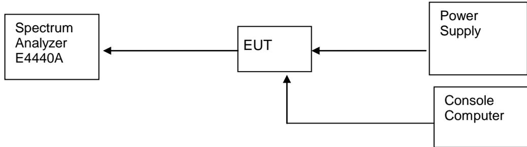
Figure 3. Test Set-up
