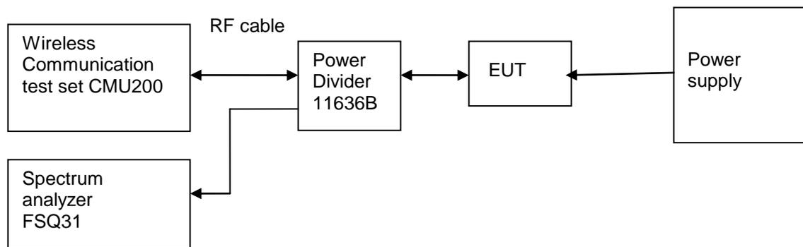
Figure 6. Test Set-up
