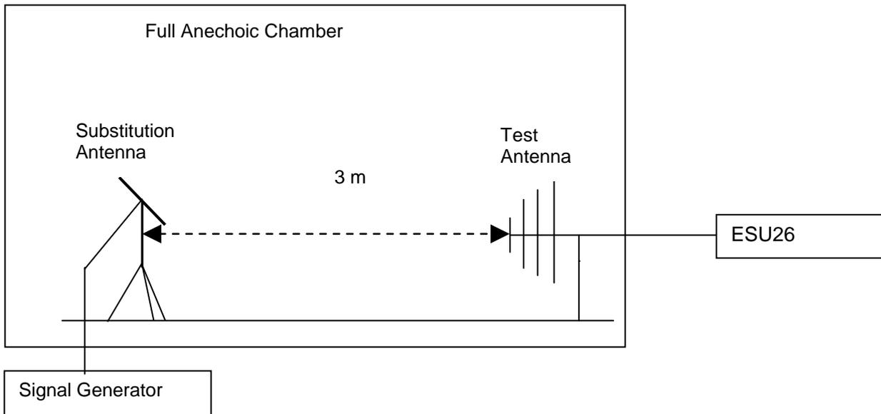
Figure 1. Test Set-up
