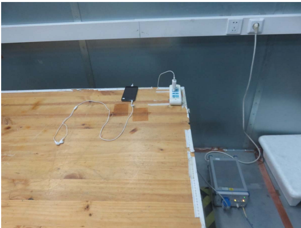
Picture 2 Conducted Emission Test Setup
