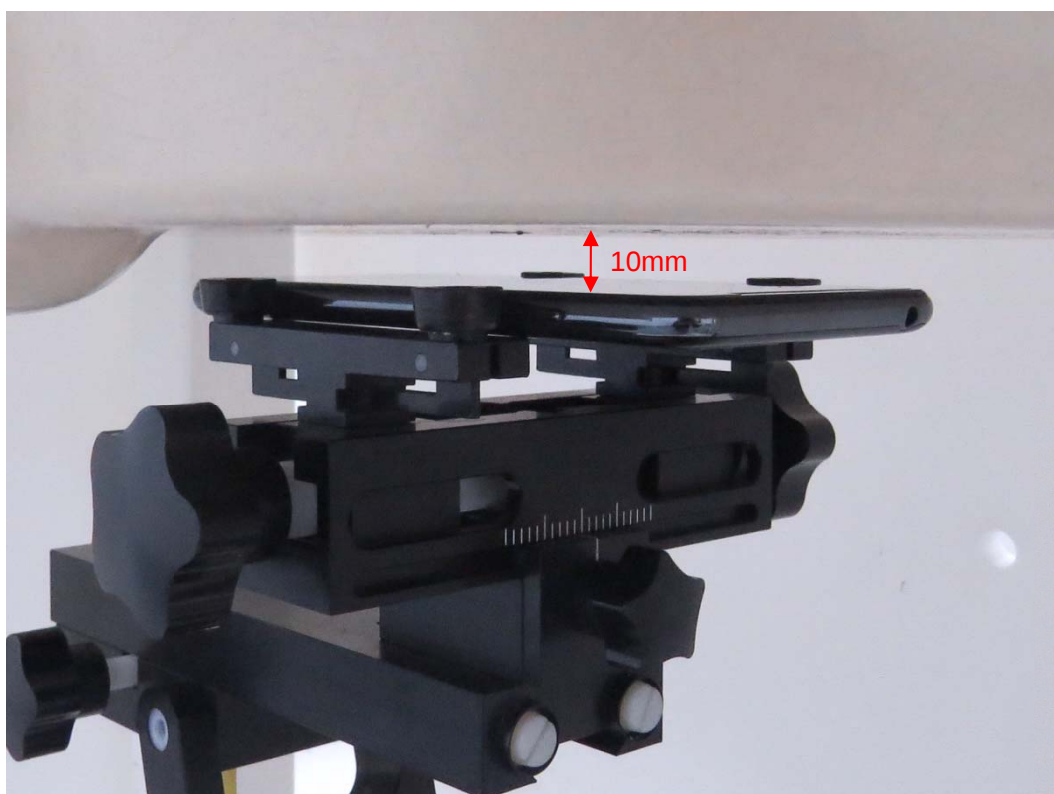
Picture 8: Front Side, the distance from handset to the bottom of the Phantom is 10mm (ATU-L11)
