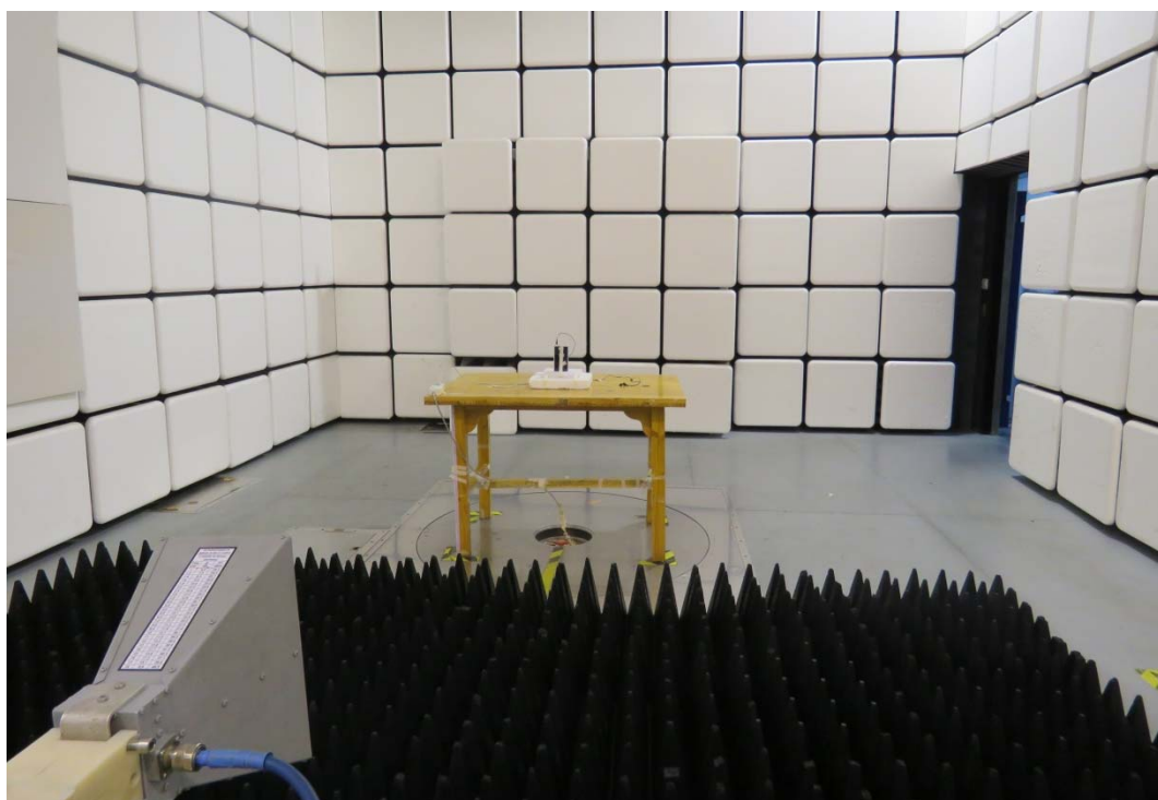
Picture 1: Radiated Spurious Emissions Test setup
