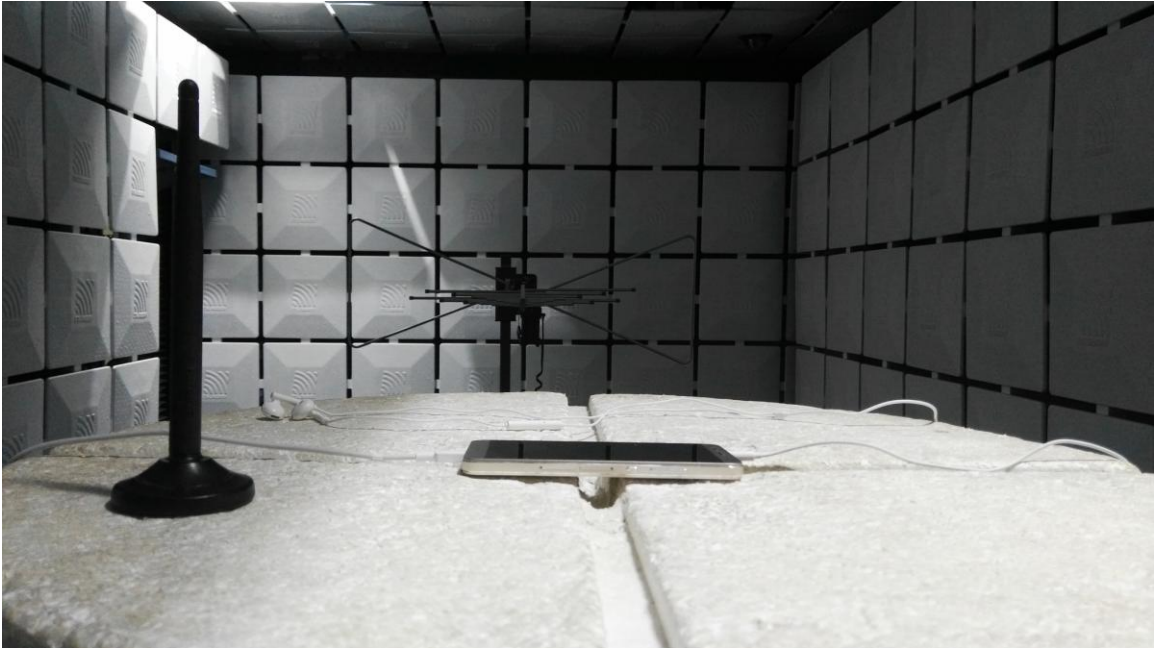
Radiated Spurious Emission (below 3GHz)
