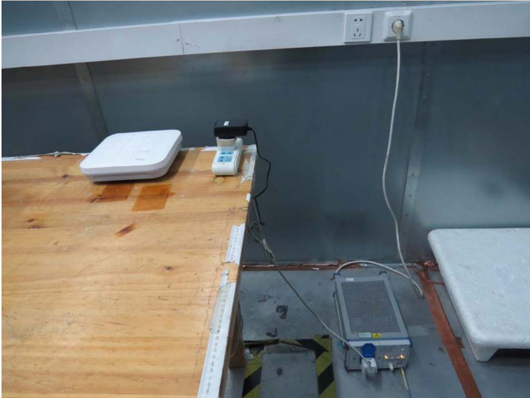
Picture 3 Conducted Emission Test Setup
