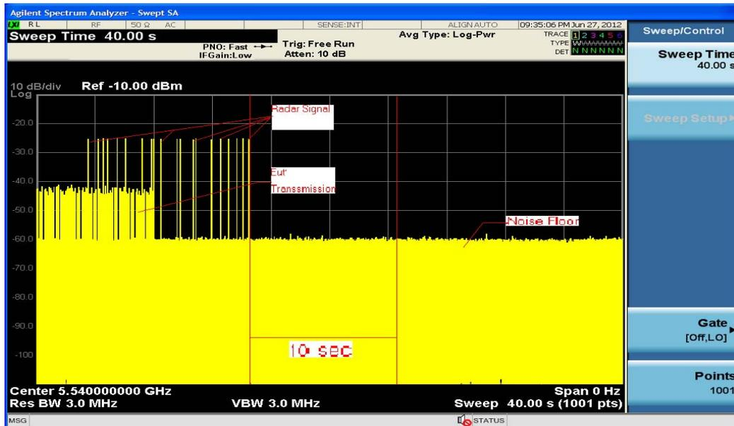
**Note:** An expanded plot for the device vacates the channel in the required 500ms
