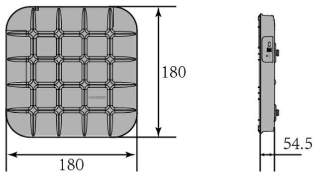
Figure 2-2 Mounting an AP (Unit: mm)
