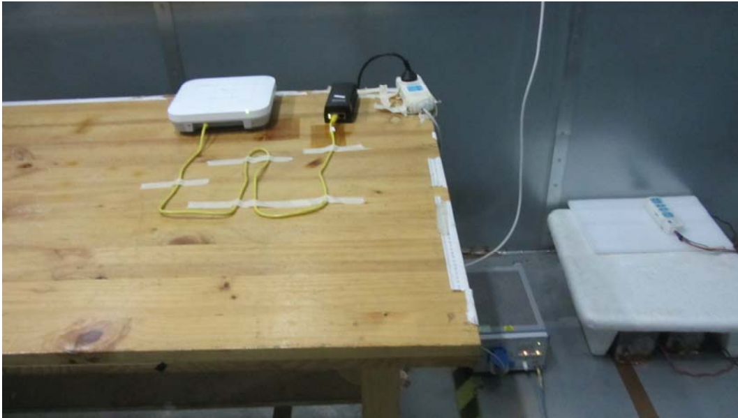
Picture 3 Conducted Emission Test Setup
