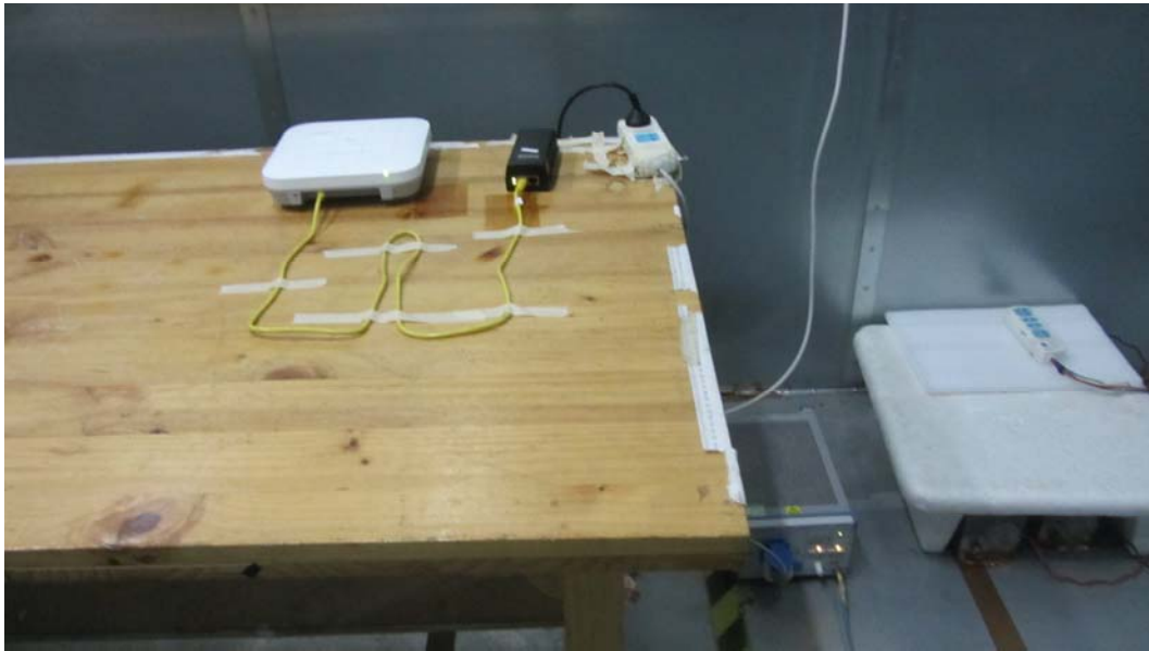
Picture 3 Conducted Emission Test Setup
