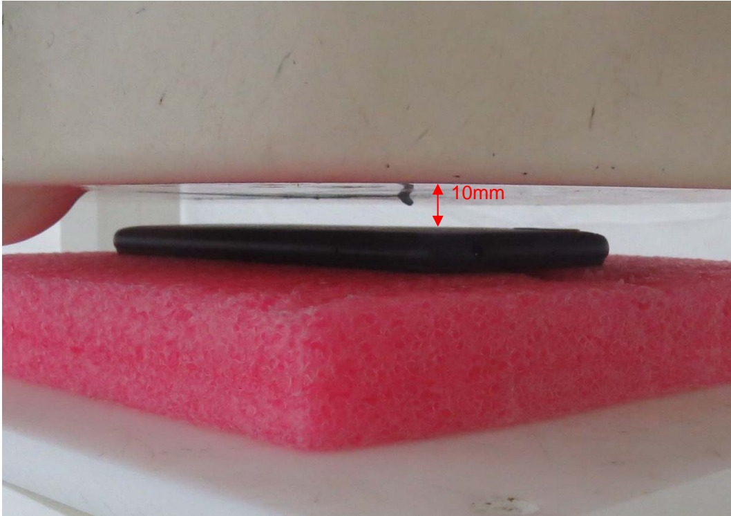
Picture 7: Back Side, the distance from handset to the bottom of the Phantom is 10mm
