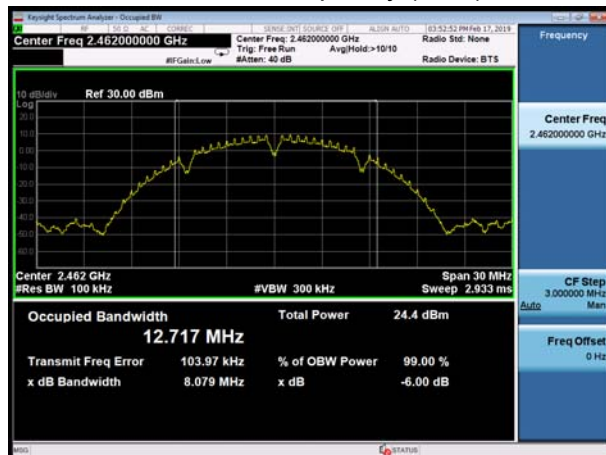
802.11b, Carrier frequency (MHz): 2462
