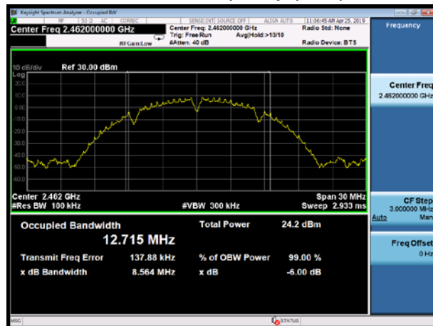
802.11b, Carrier frequency (MHz): 2462
