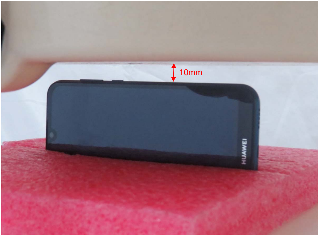
Picture 11: Right Side, the distance from handset to the bottom of the Phantom is 10mm
