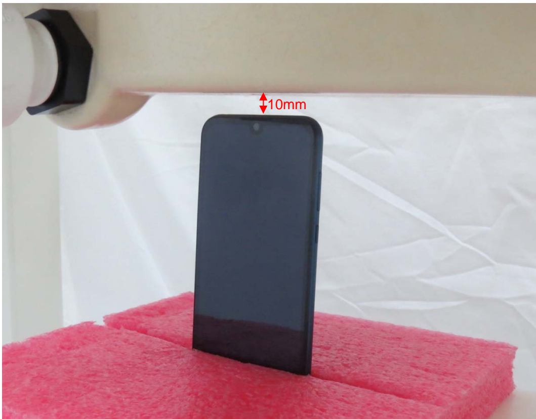
Picture 12: Top Side, the distance from handset to the bottom of the Phantom is 10mm
