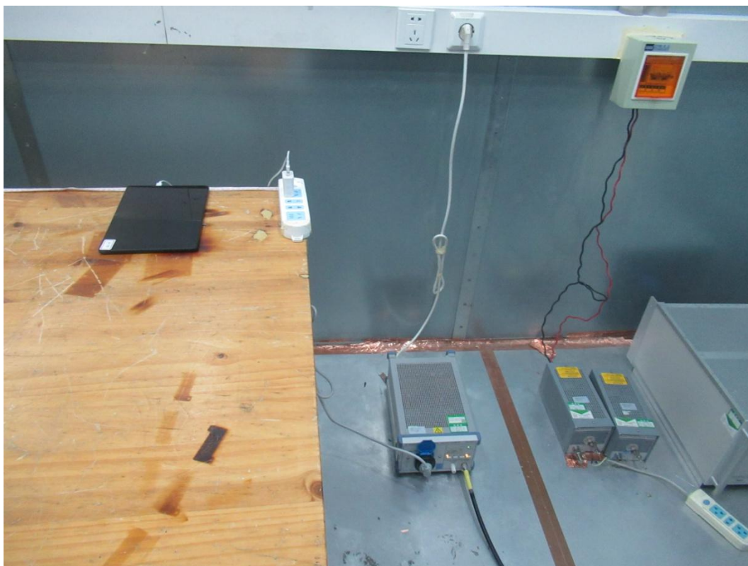
Picture 2 Conducted Emission Test Setup
