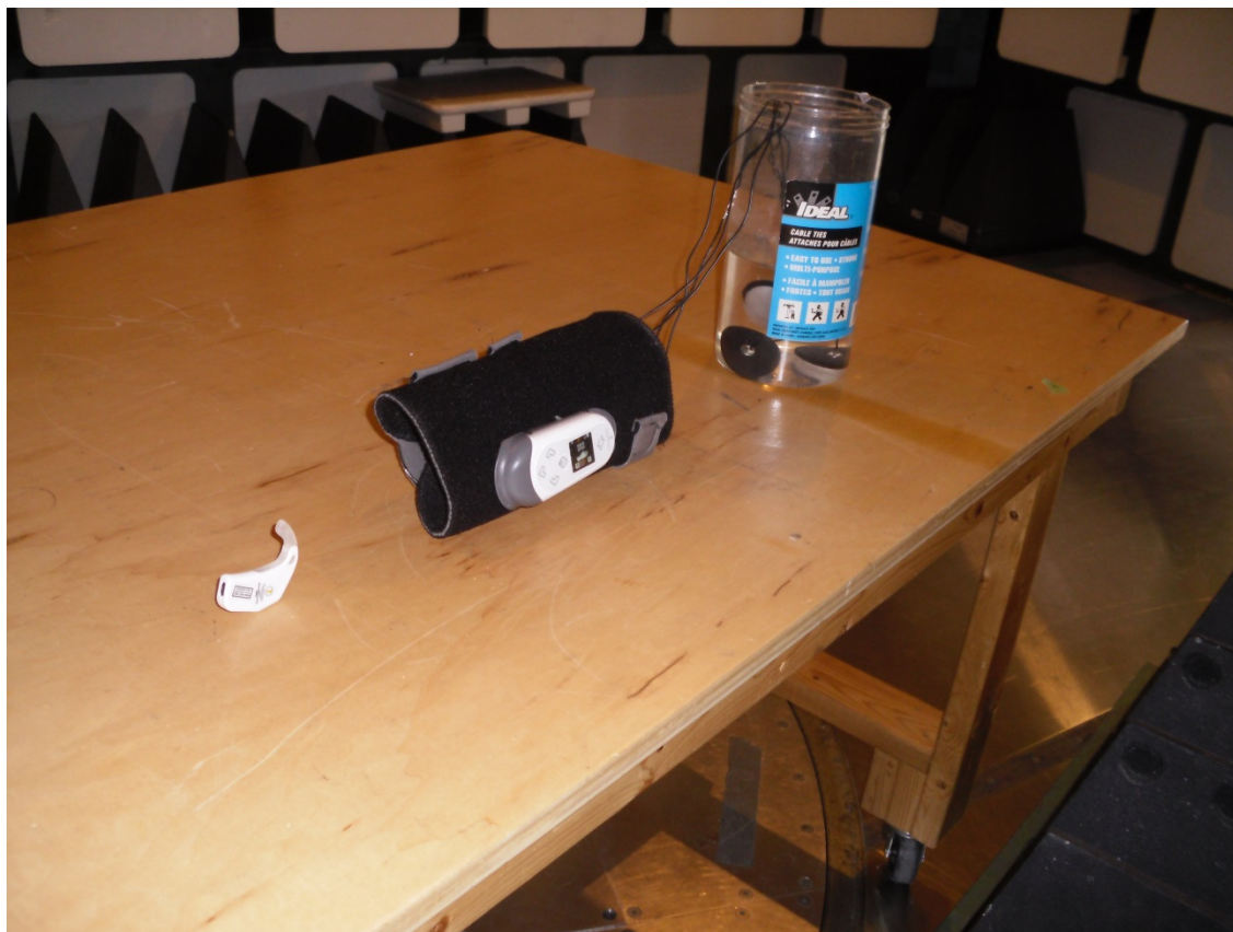
Hand Stimulator with HMS unit, Garment and Electrodes in Saline solution
