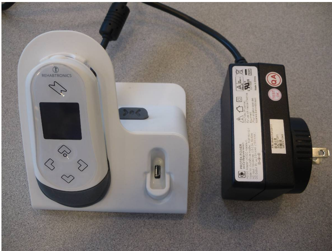
Hand Stimulator with AC/DC Power supply adaptor and Charge Dock
