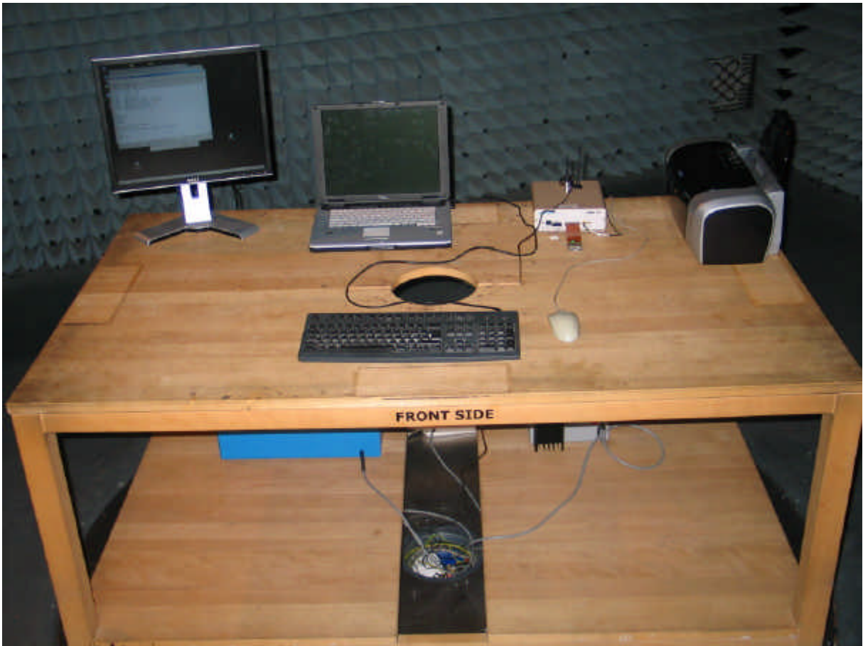
Photo 2: Test setup for radiated measurements
