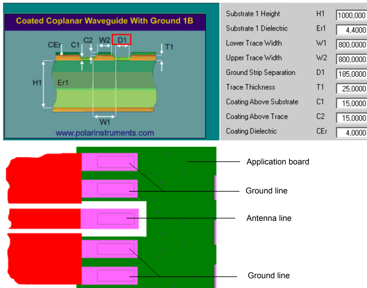
Figure 7: Micro-Stripline on 1.0mm standard FR4 2-layer PCB - example 1
