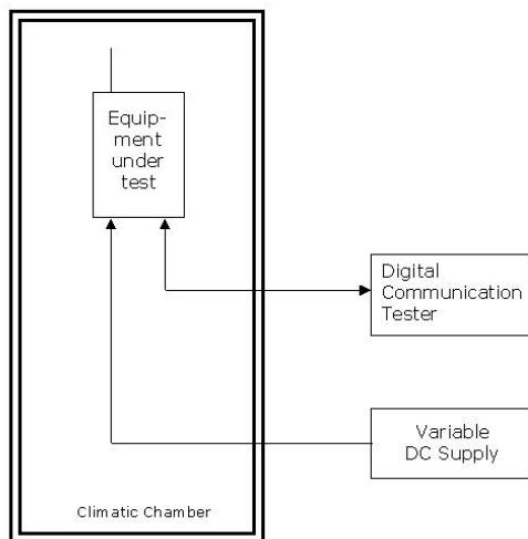
Principle set-up for tests under extreme test conditions
