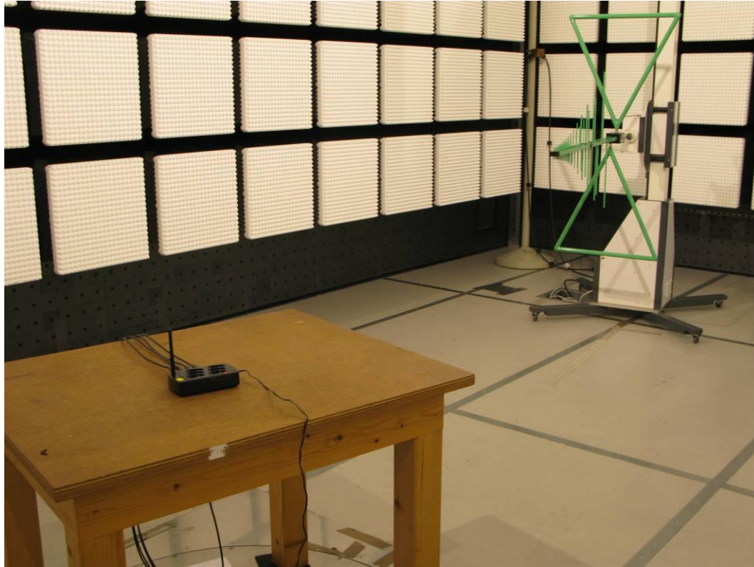
Photograph 1: - AW-A Wireless base station, test setup radiated emissions (30 - 1000 MHz)
