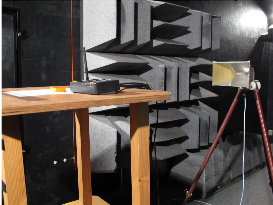
Photograph 2: - AW-A Wireless base station, test setup radiated emissions (1 - 18 GHz)
