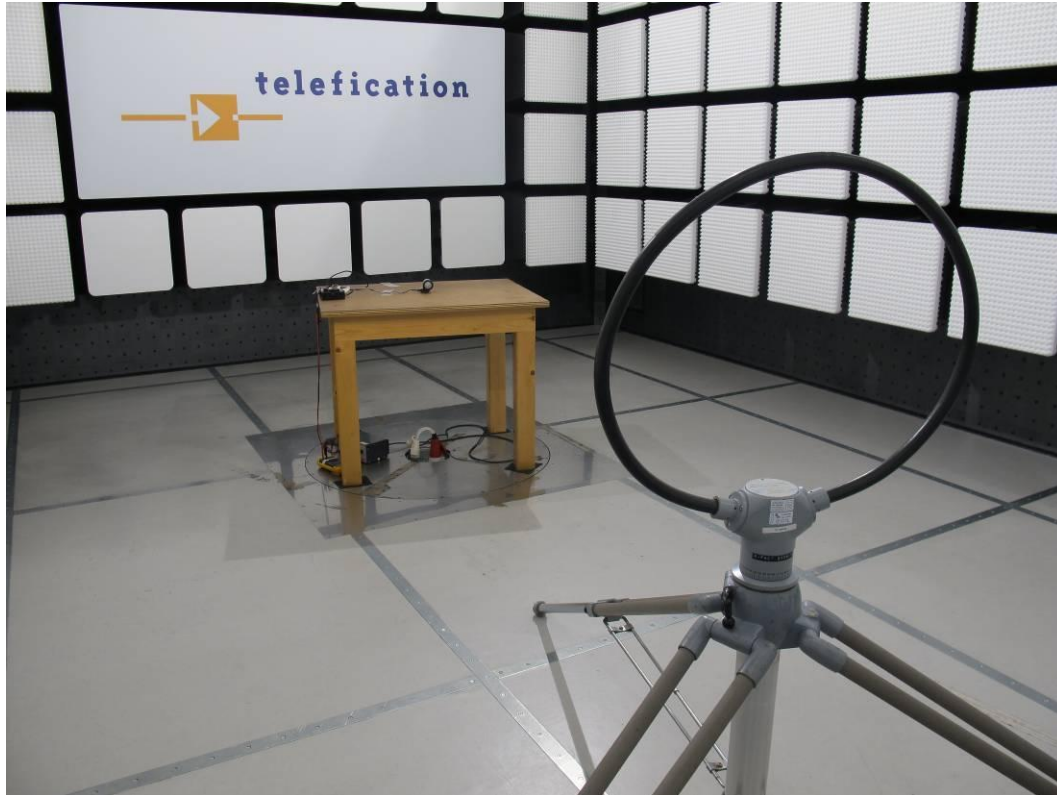
Photograph 1: - Radiated emissions test set up, 0.15 – 30 MHz
