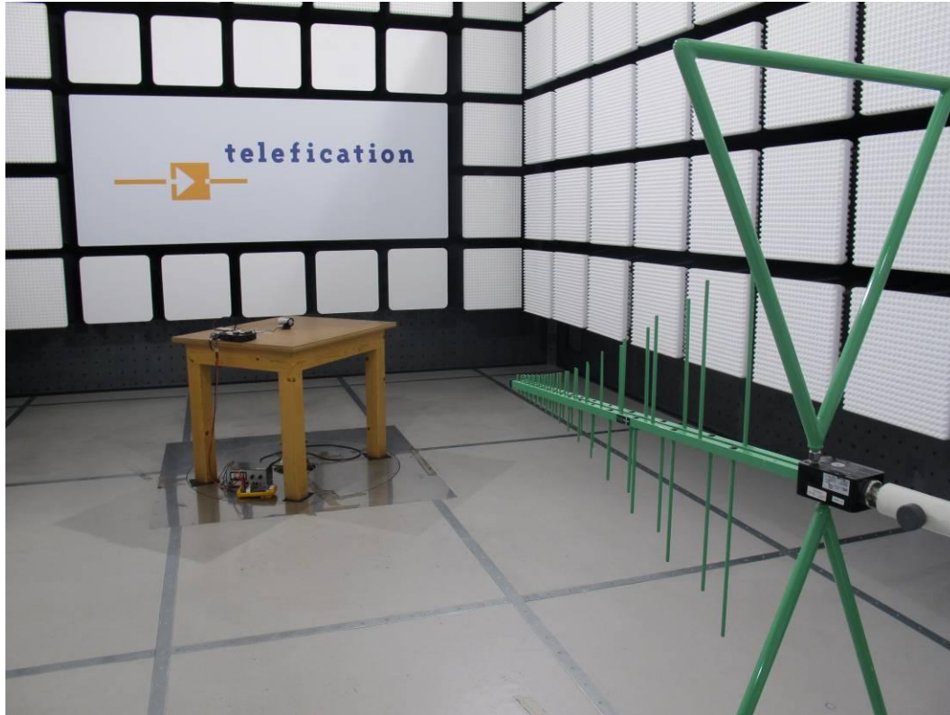
Photograph 3: - Test setup radiated emissions (0.03 - 1 GHz)
