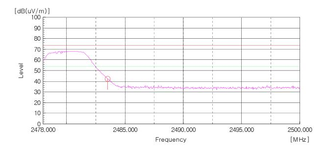
AV Detector: RBW: 1MHz, VBW: 10 Hz (2 483.5 MHz - 2 500.0 MHz), Worst case (High, Horizontal)
