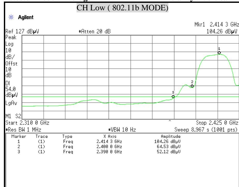
**Detector mode : Peak****Polarity : Horizontal**
