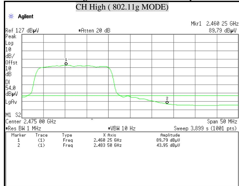
**Detector mode : Peak****Polarity : Vertical**
