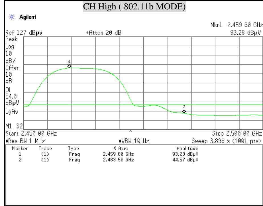
**Detector mode : Peak****Polarity : Vertical**
