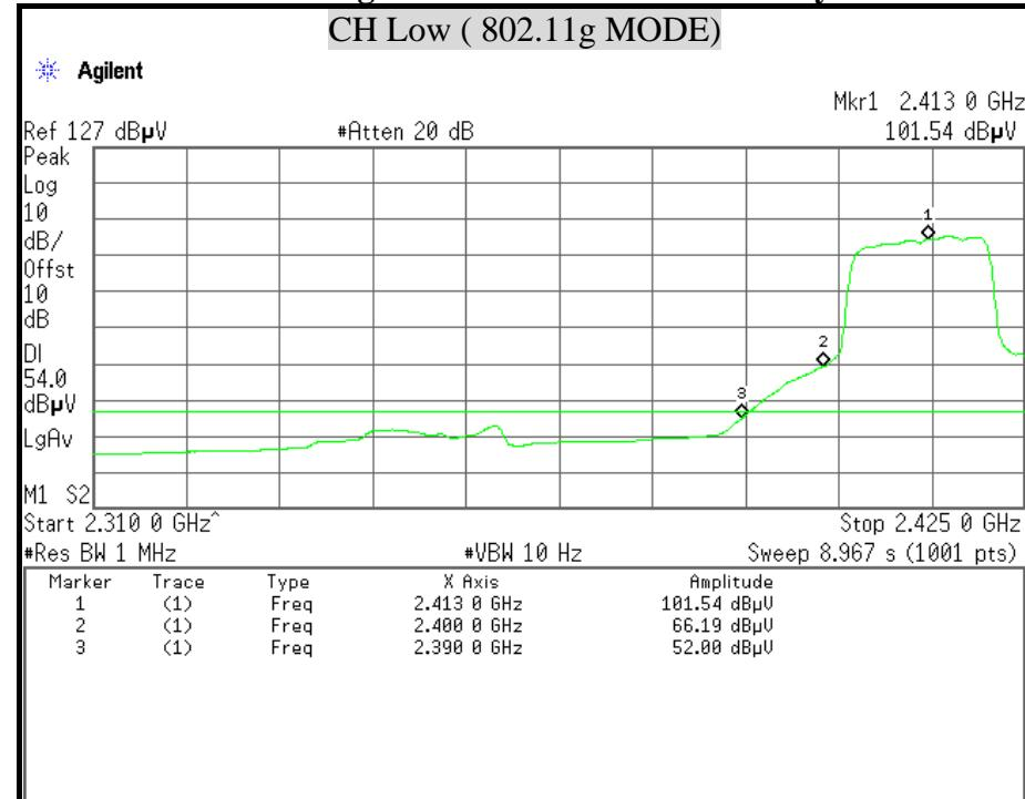
**Detector mode : Peak****Polarity : Horizontal**
