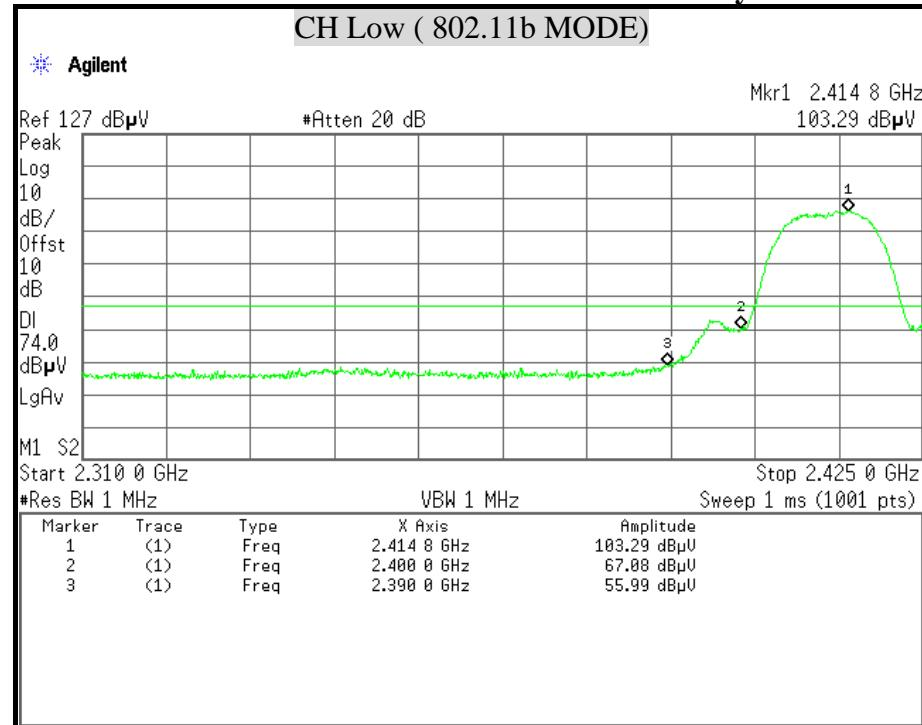
**Detector mode : Average****Polarity : Horizontal**
