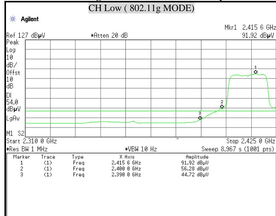
**Detector mode : Peak****Polarity : Vertical**
