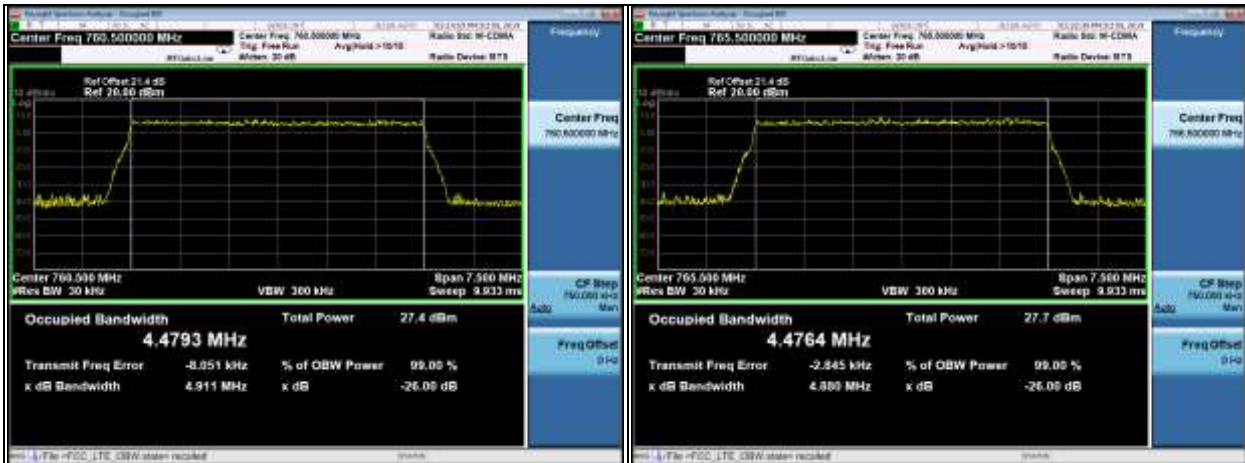
5MHz, QPSK, Low Channel
