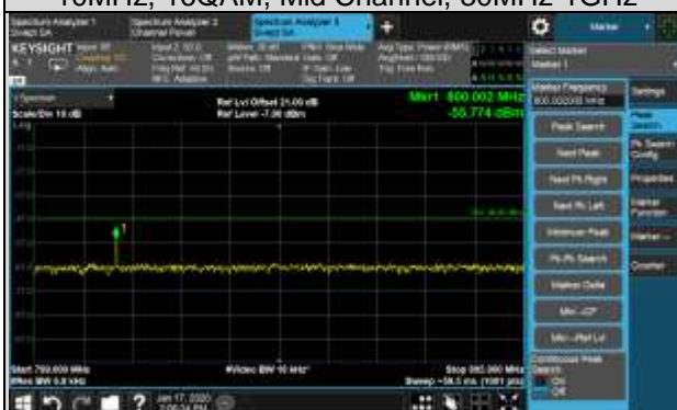
10MHz, 16QAM, Mid Channel, 769MHz-775MHz
