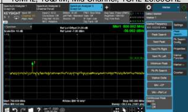
10MHz, 16QAM, Mid Channel, 799MHz-805MHz
