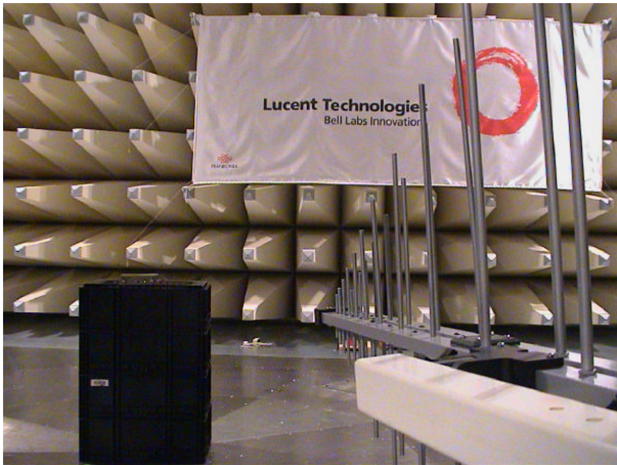
Fig. 2: Basic set-up for radiated and spurious emission; 30 MHz - 1 GHz
