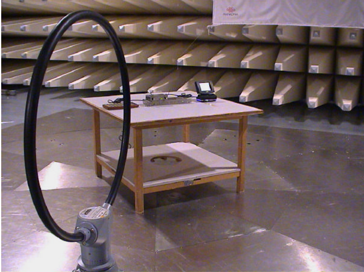
Fig. 1: Basic set-up for radiated emission; 9 kHz - 30 MHz
