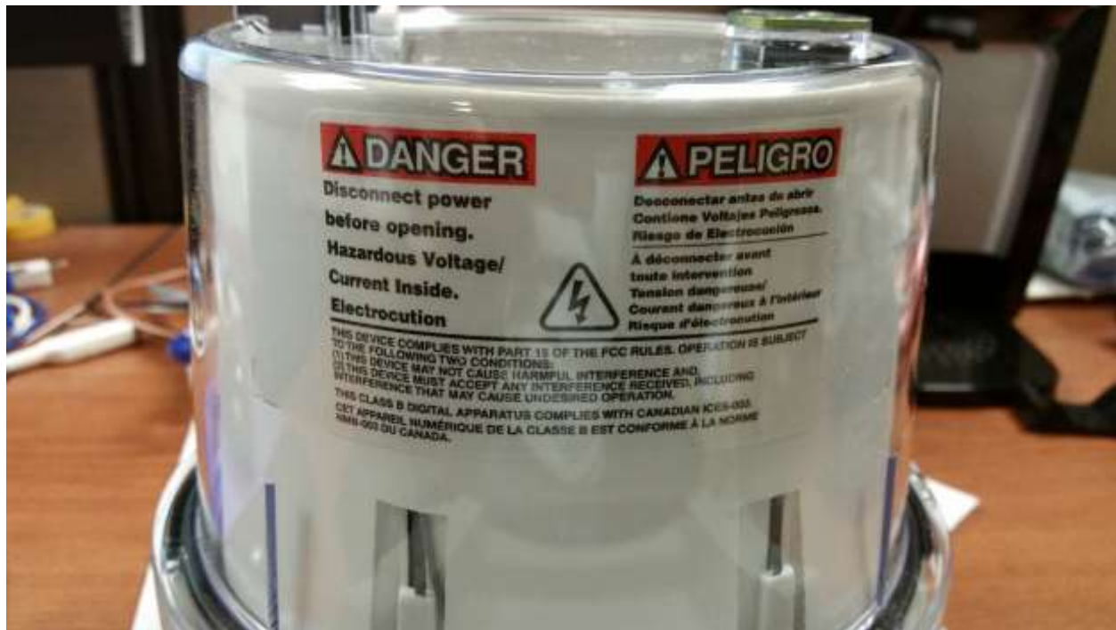
FCC & IC COMPLIANCE LABEL ON HOST METER
