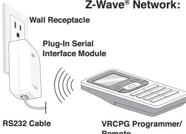
**NOTE:** Programmer/Remote must be in close proximity (approx. 1 foot) to Plug-In Serial Interface Module when including into network
