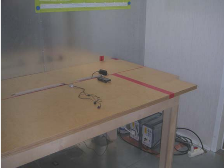
Picture 3 AC powerline conducted emission measurement
