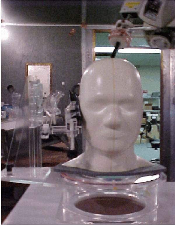
Figure S15. Configuration #15 - Cheek ( 0^{\circ} ) position, left side, GPS In, 900 mAH Battery
