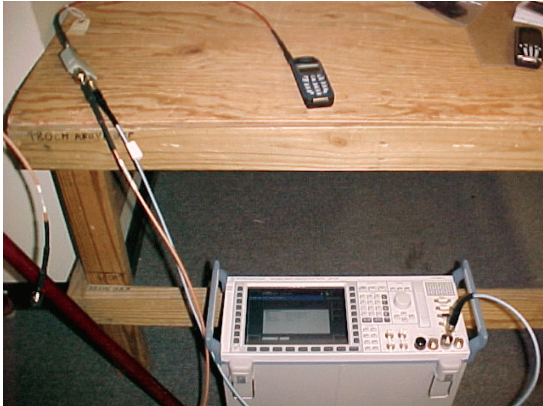
Figure 2. Photograph of Part 24 Tests Setup
