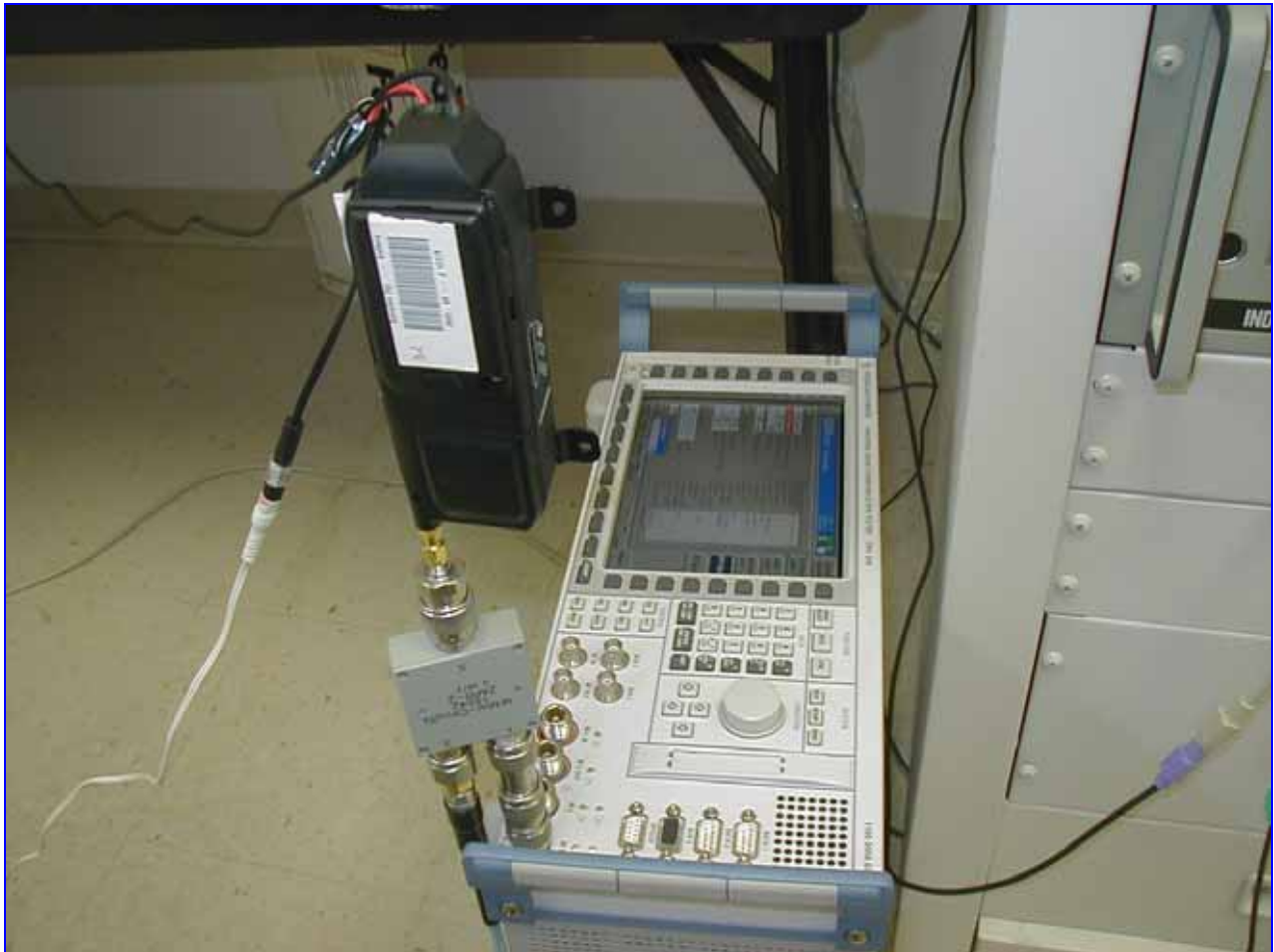
Photograph 1. EUT Test Setup Photos for Part 24 - Broadband PCS Devices
