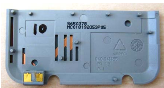
Fig 10 –Antenna module/cover: rear view (Integral 850/900/1800/1900 antennas)
