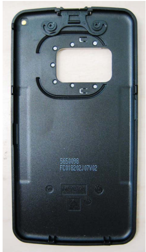
Fig 12 – Battery cover rear view (integral BT/WLAN/GPS/DVB-H antenna)
