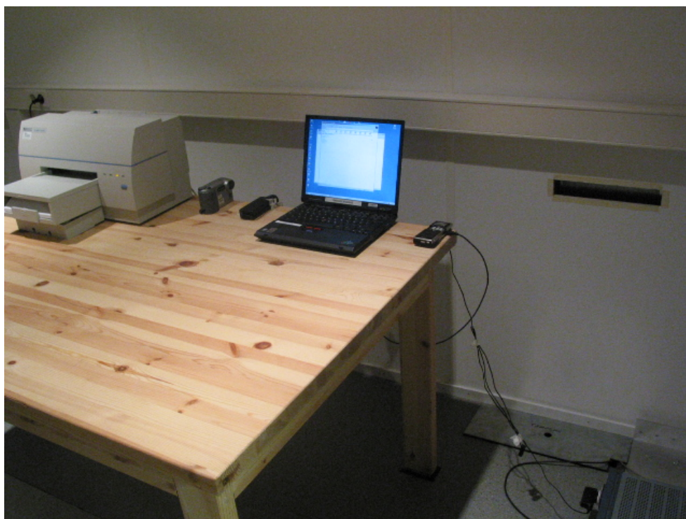
Picture 5 AC powerline conducted emission measurement (WLAN)
