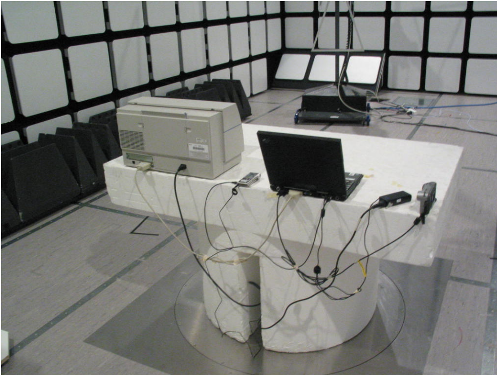
Picture 3 Radiated emission measurement (WLAN)
