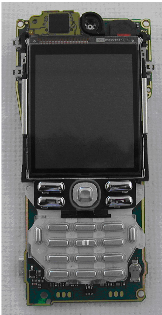
Fig 3 – PCB – Front View with Display and keymat
