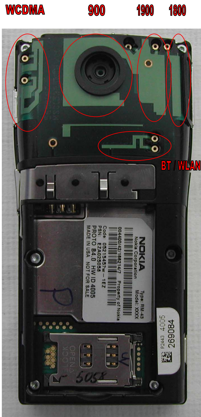
Fig 6 – Back showing antennas
