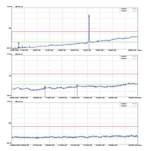
Page 79 Rev. 00 Operation Mode: Tx / IEEE 802.11n HT 20 MHz Channel
