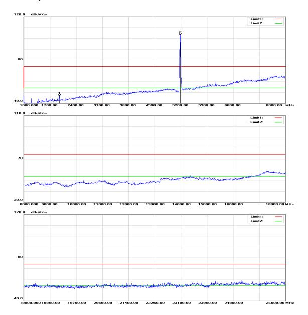
Page 55 Rev. 00 Operation Mode: Tx / IEEE 802.11n HT 20 MHz Channel
