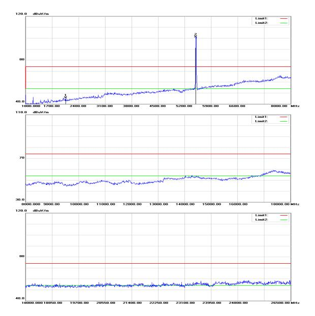
Page 94 Rev. 00 Operation Mode: Tx / IEEE 802.11a mode / 5500 MHz Test Date: August 19, 2015
