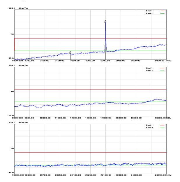
Operation Mode: Tx / IEEE 802.11n HT 20 MHz Channel
