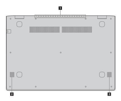
1 Ventilation slots Dissipate internal heat.
