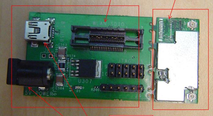
For WLAN testing the device can be power via USB or 5V DC power supply, either one is fine, and the true connector is the SDIO interface. For BT& BLE, USB is required for connection and power(without SDIO connection).
