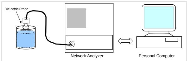
Set-up for liquid parameters check
