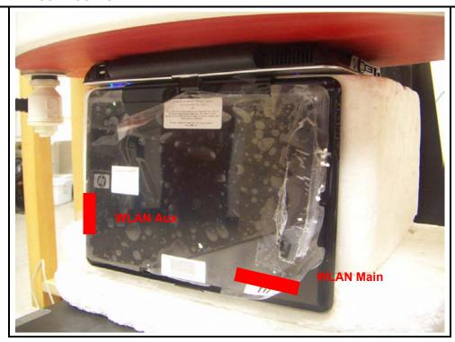
This position was skipped due to larger distance between the antennas and the phanton
