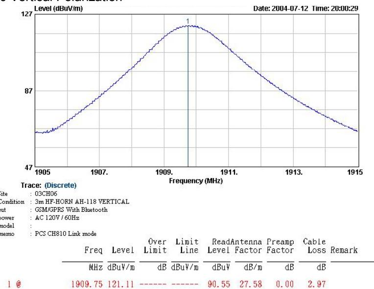
**Name of Test:** Emission Masks (Occupied Bandwidth)
