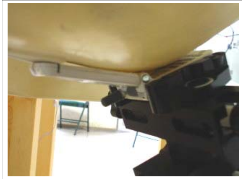
EUT Setup Configuration 2 (Right Head - Touched position)
