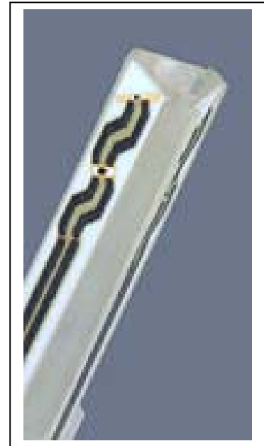
Inside view of ET3DV6 E-field Probe
