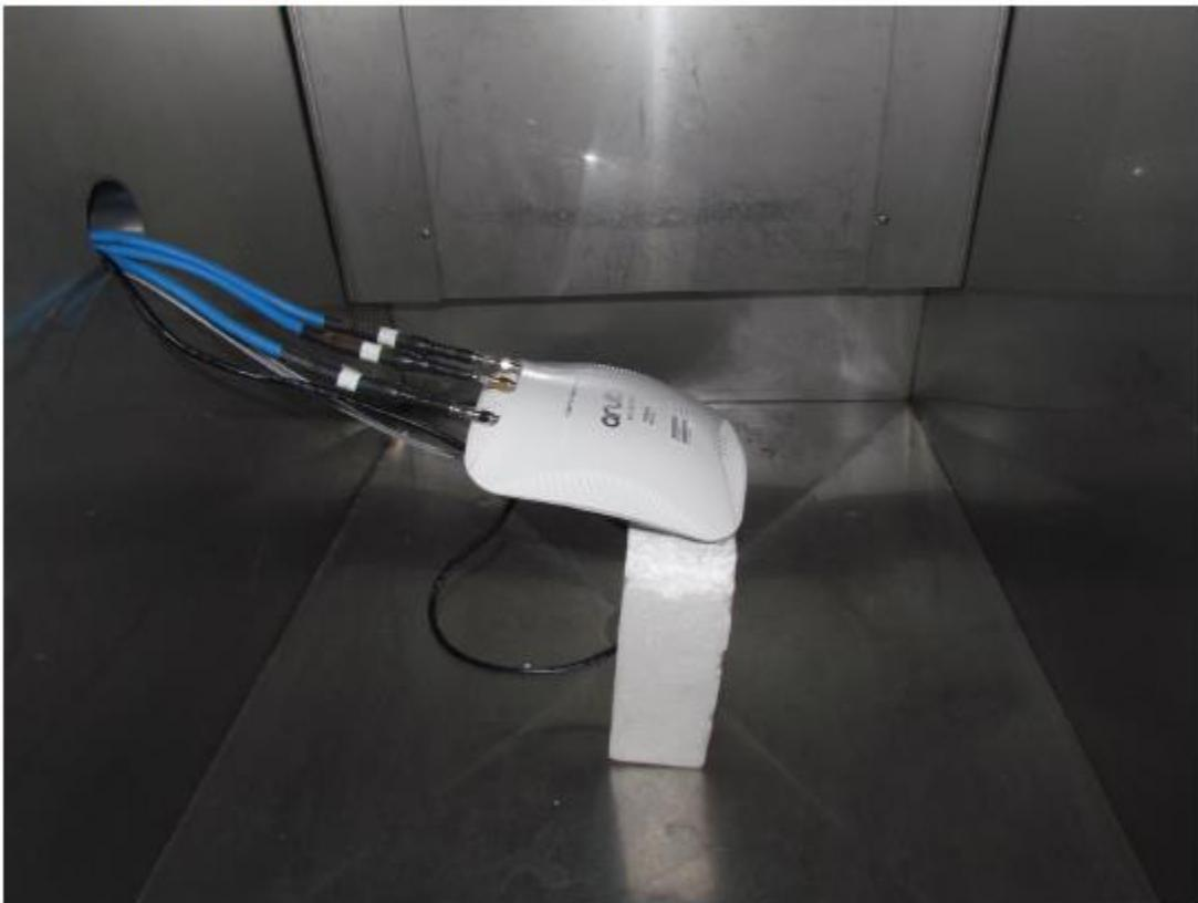
**Test Setup - Digital Emissions > 1 GHz**
