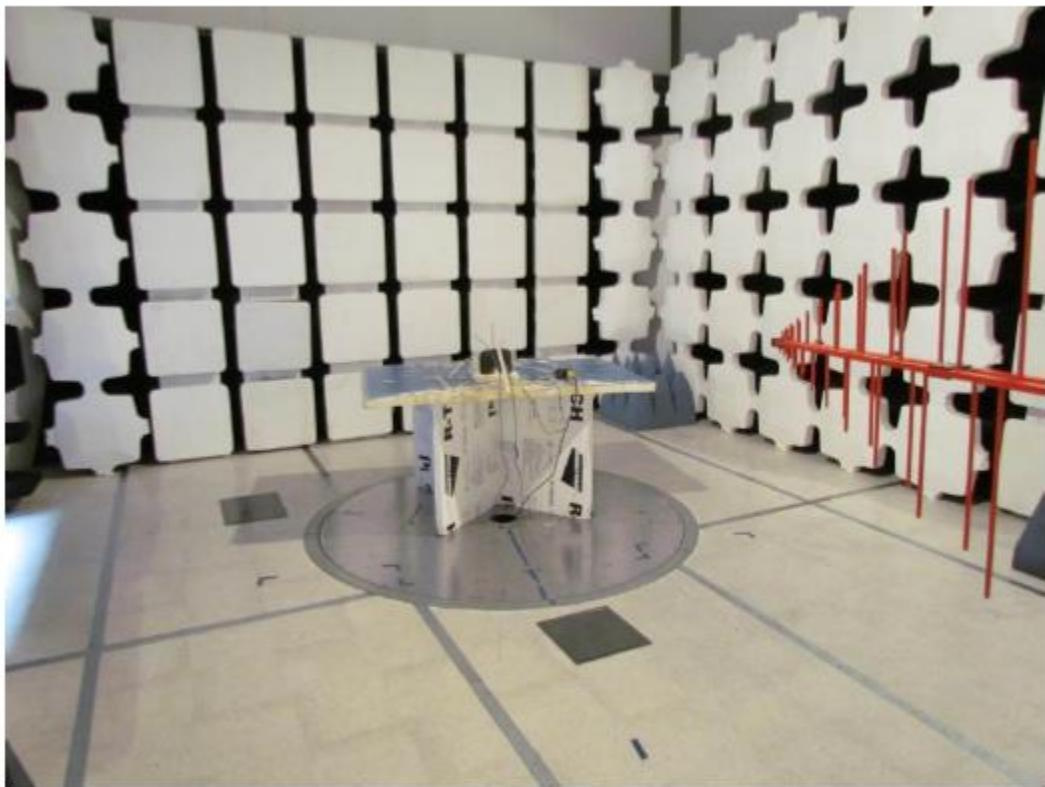
**ac Wireline Test Setup >1 GHz**
