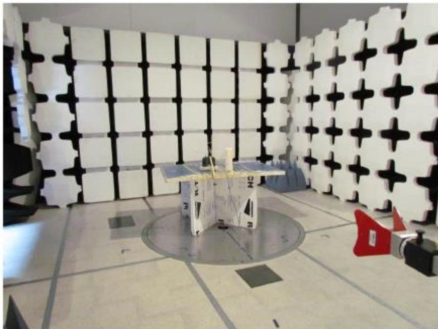
**6.3. Radiated Emissions Test Setup <1 GHz**
