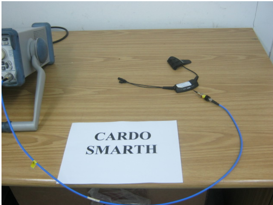
Figure 5. Conducted Emission From Antenna Ports Test
