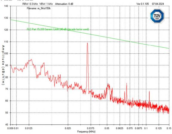
Note: Emission shown at 35 kHz was ambient signal.
