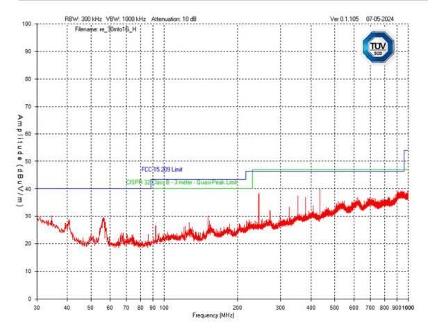
Note: testing was performed to 10 GHz, no emissions above 1 GHz were detected and the reading were below the applicable limit(s).
