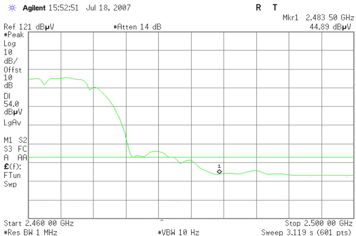
**Band Edges (IEEE 802.11g / CH Low)****Detector mode: Peak****Polarity: Vertical**
