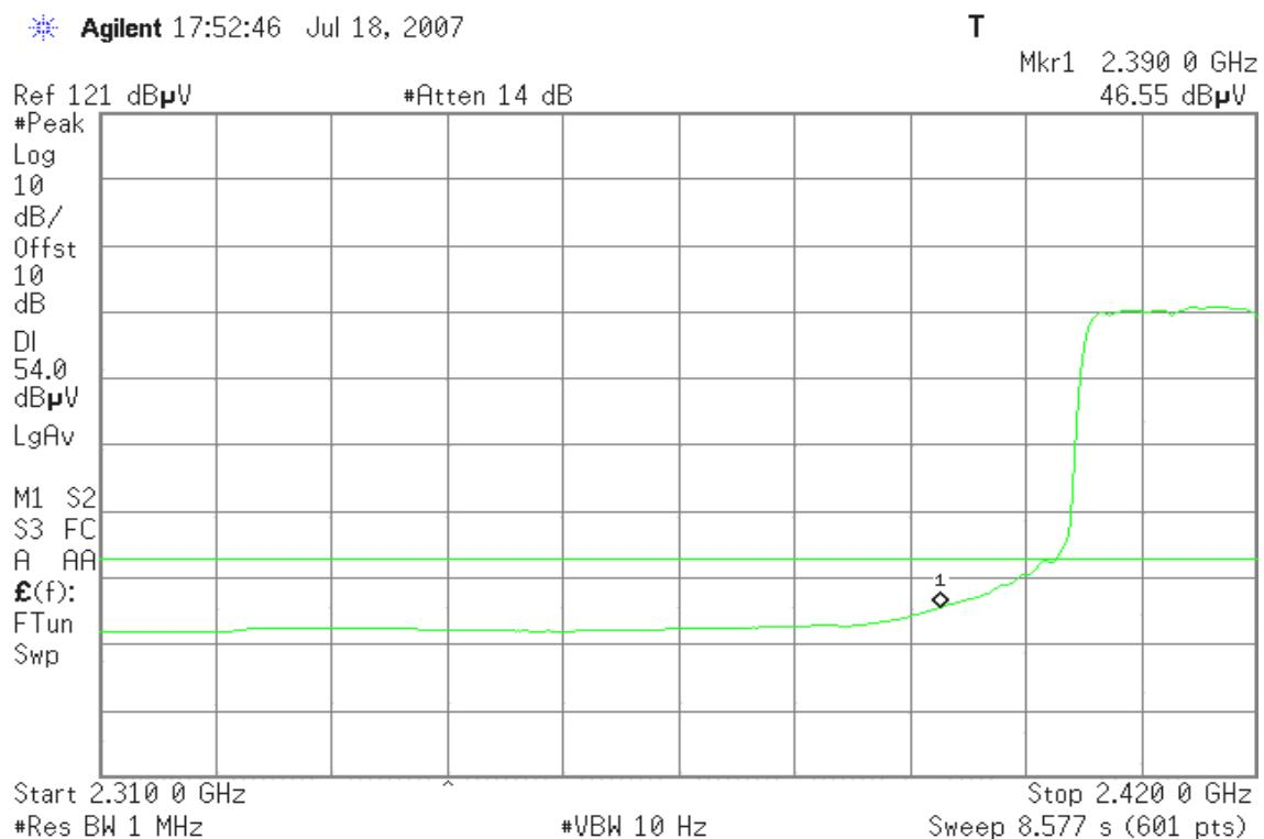
**Band Edges (IEEE 802.11g / CH High)****Detector mode: Peak****Polarity: Vertical**
