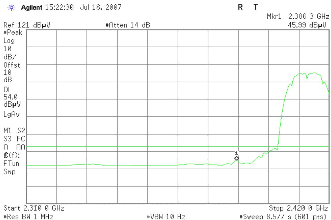
**Band Edges (IEEE 802.11b / CH High)****Detector mode: Peak****Polarity: Vertical**
