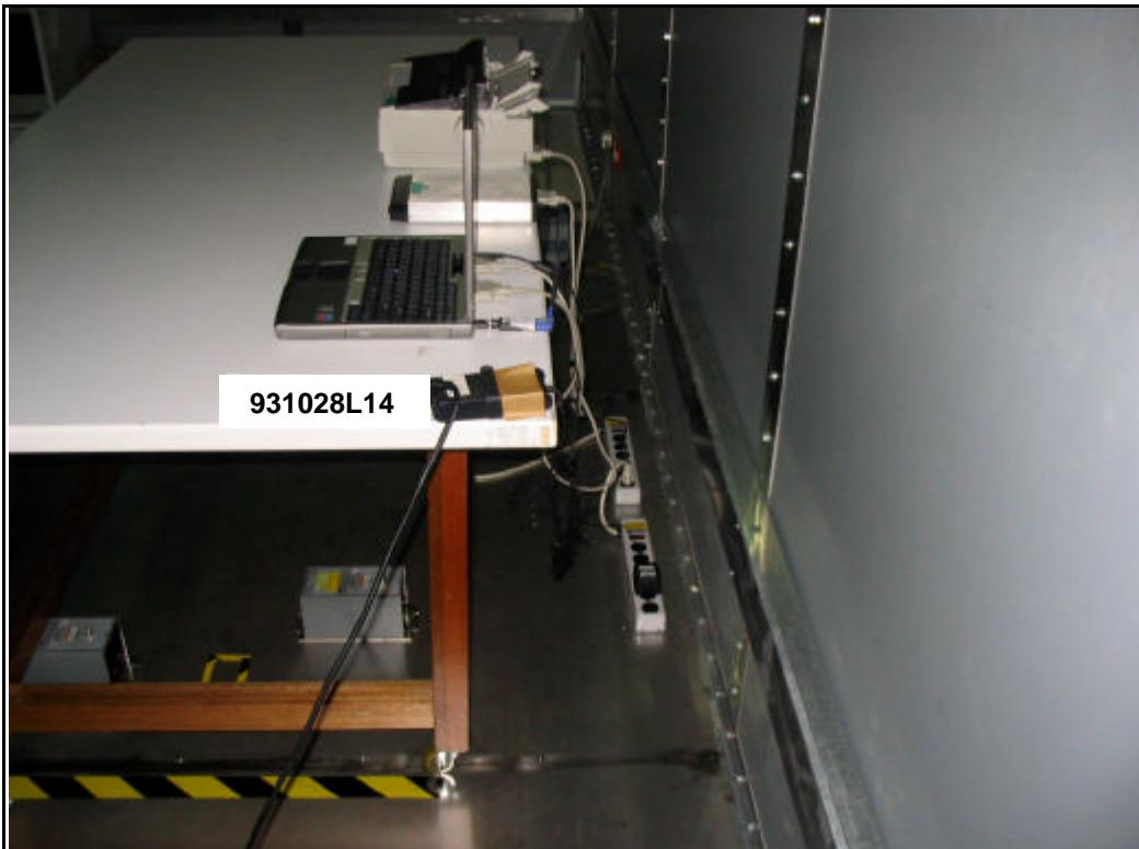
CONDUCTED EMISSION TEST (TEST MODE 2)
