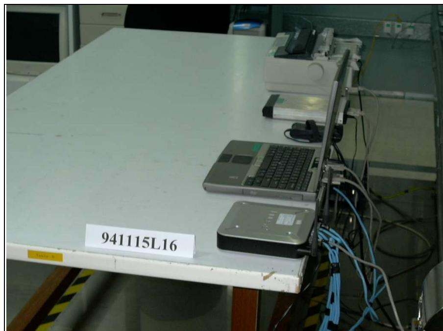
CONDUCTED EMISSION TEST (TEST MODE B)
