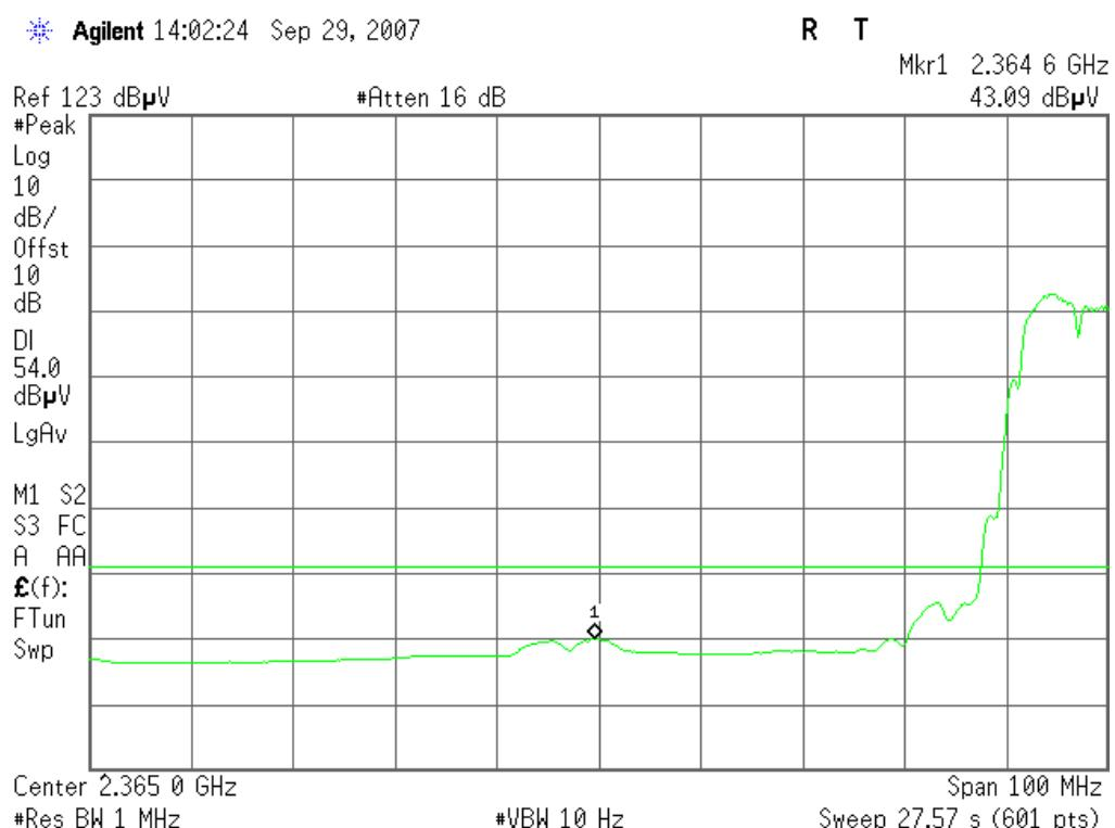
**Band Edges (IEEE 802.11b mode/ CH 11)****Detector mode: Peak****Polarity: Vertical**
