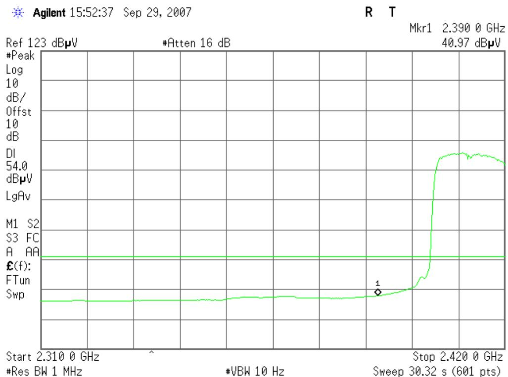
**Band Edges (IEEE 802.11g mode / CH 11)****Detector mode: Peak****Polarity: Vertical**
