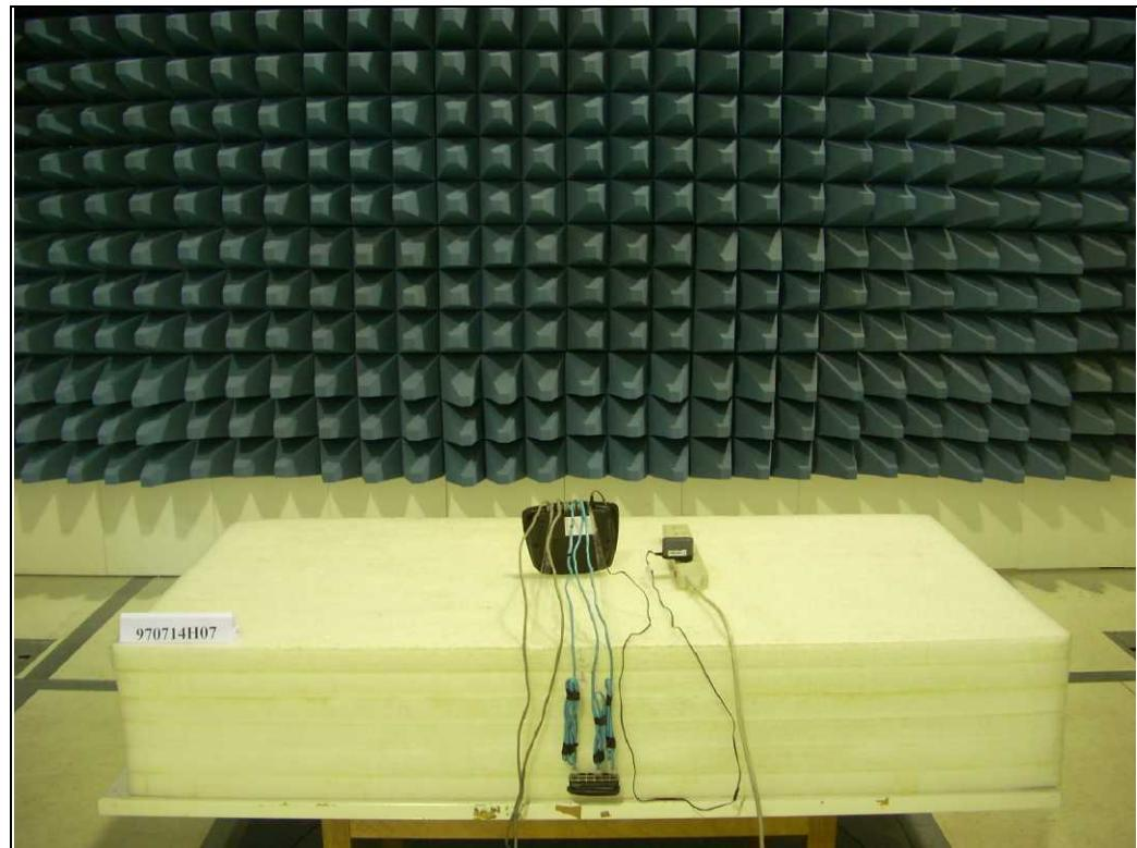
**RADIATED EMISSION TEST – below 1GHz (Mode 3)**
