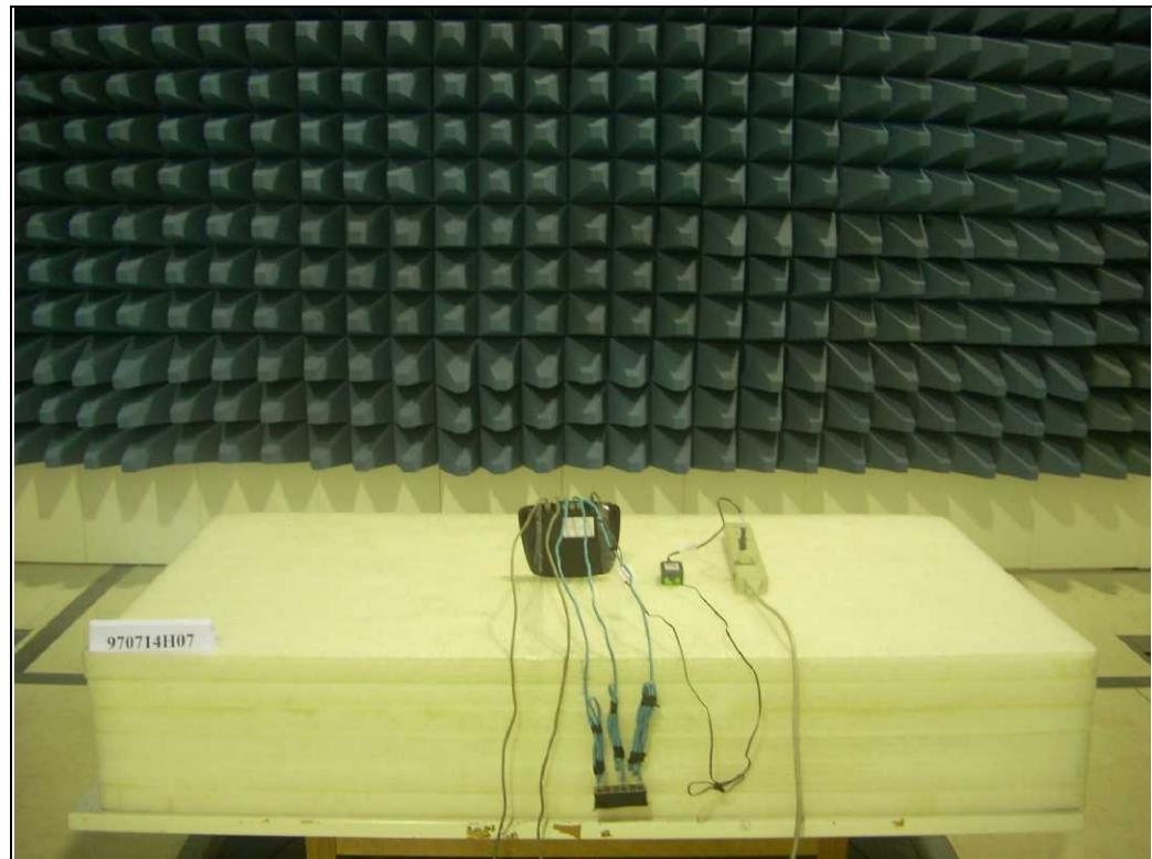
**RADIATED EMISSION TEST – below 1GHz (Mode 2)**
